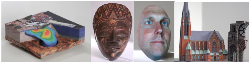
Figure 2. Examples of full-color 3D printed models from the Mcor Iris paper-based printer. For more images, see http://mcor technologies.com/3d-printers/iris/
